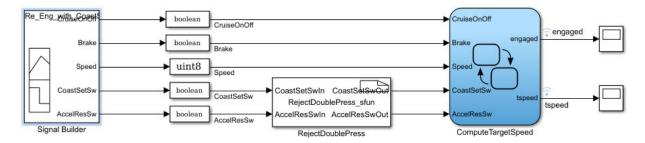
The model is a cruise control system that consists of test cases and input signals from a Signal Builder block. The signals from the Signal Builder act as inputs to the Stateflow chart ComputeTargetSpeed, which engages or disengages the cruise control system and sets the target speed, tspeed.
