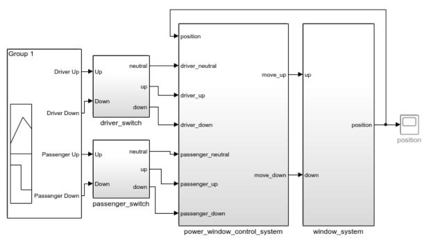
Simulink Coverage Power Window Controller Hybrid System Model
