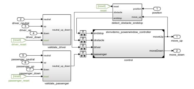
The slvnvdemo\_powerwindow example model opens, showing the power\_window\_control\_system subsystem.
